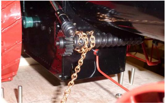
Start by putting the bolts through the last link in the steering chain, use M2 by 14 steel screws, one in each chain. Lay the engine on its side and push the
